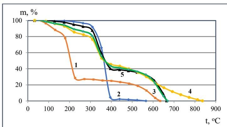
Figure 4. TGA curves for graphene oxide (*1*), melamine (*2*) and their mixtures with ratios (1:1) (*3*), (1:2) (*4*), and (1:5) (*5*)
