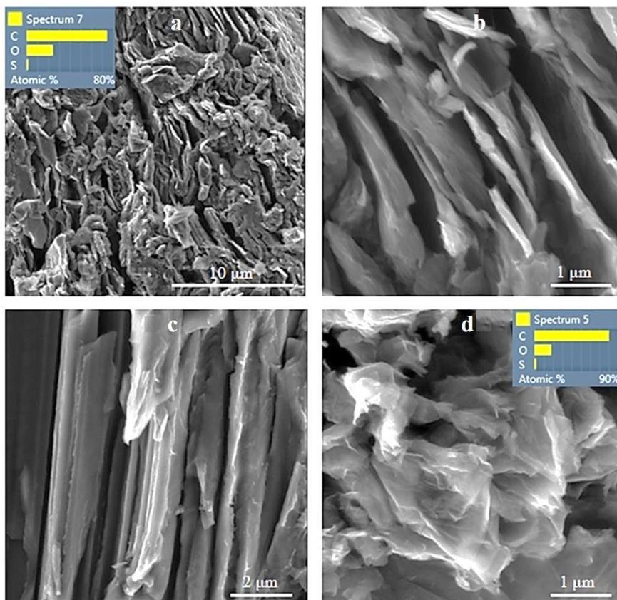
Figure 3. SEM images of synthesized GO (*a, b*) and GO+UST (*c, d*)
