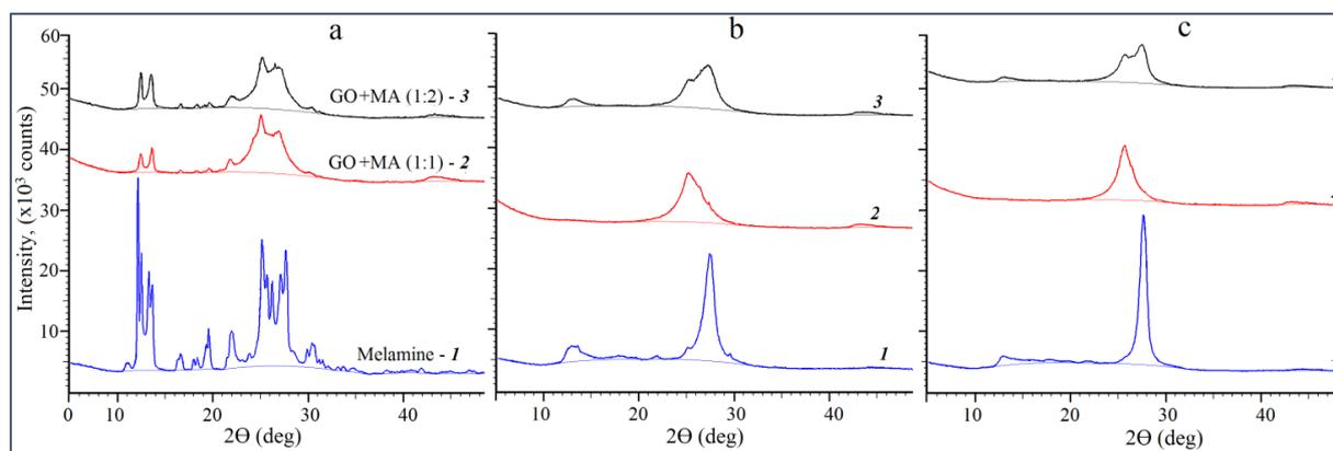
Figure 7. XRD patterns of melamine and its mixtures with graphene oxide after heat treatment at 450 °C (a), 500 °C (b) and 550 °C (c)
